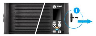
Remove the Ferodo washer fixed with two Philips countersunk head screws M4x10 black on the right side panel cover as show in the picture. You can identify the "right side" because is where the display and tactile buttons are located.
