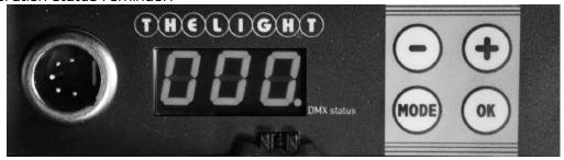
Use DMX XLR-5 in&out splitter cables (ref. THE-VL-DMXinout) to daisy chain several VELVET panels or mix them within any DMX line of different fixtures.
