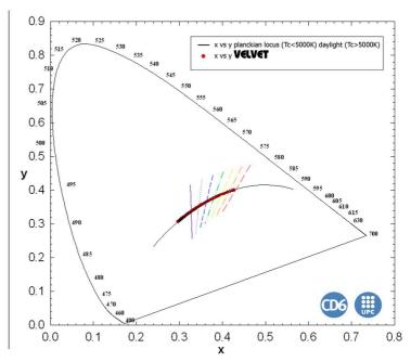
Shown on the diagram are the VELVET lamp head chromaticity coordinates (x, y CIE-1931) feed and digitally controlled by its Control Unit and they are compared with the reference illuminants. These reference illuminants are the Planckian locus radiator set below 5000K and the CIE daylight reference is set over 5000K. The Planckian locus radiator references the chromaticity for several tungsten lamps colour temperatures while the daylight locus typify daylight type D illuminants.
