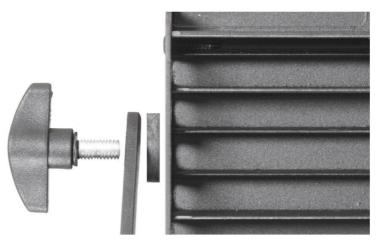
Assemble the Yoke to the LED panel by using the mounting kit of bolts, washers and adjustable handle. First mount the handles with the metric M8 metal washer then insert the thick rubber washers between the Yoke and the LED panel.
